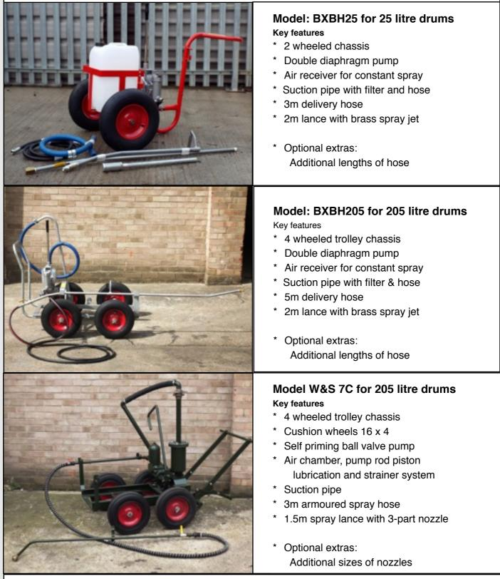
Direct from drum hand-operated sprayers for use with 25 or 205 litre drums of cold bitumen emulsion
